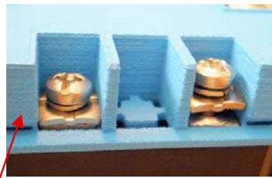
M4 control connection
