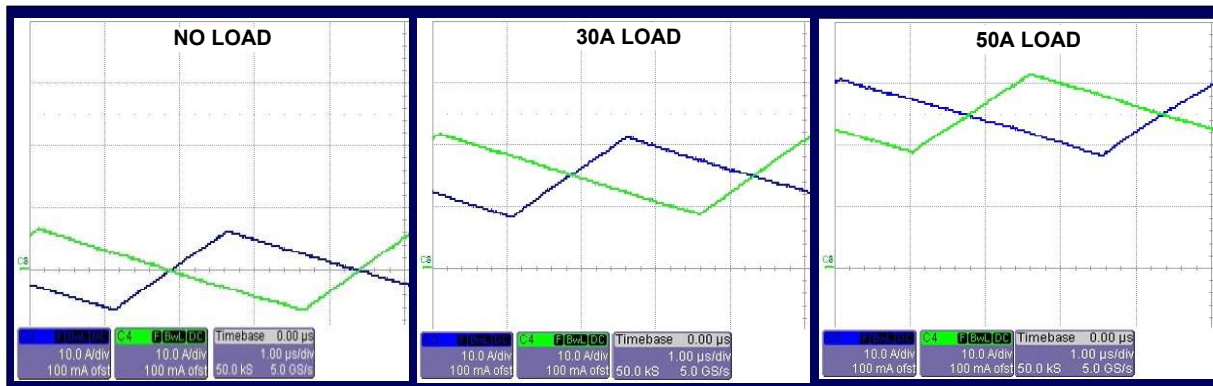
FIGURE 12. INDUCTOR CURRENT WAVEFORMS
