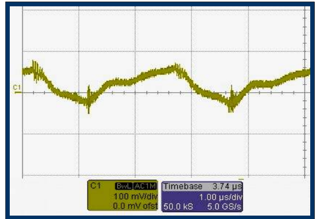
FIGURE 26. OUTPUT VOLTAGE RIPPLE, 20MHZ (SP101)
