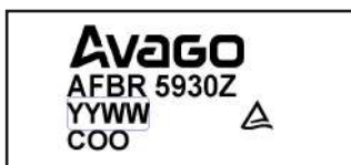
Figure 2b. Component Labeling information
