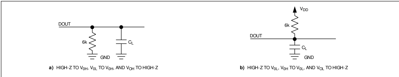
Figure 1. Load Circuits for Enable and Disable Time
