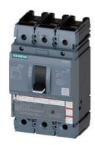
circuit breaker 3VA5 UL frame 250 breaking capacity class H 65kA @ 480 V 3-pole, line protection TM210, FTFM, In=90A overload protection Ir=90A fixed short-circuit protection Ii=10 x In nut keeper kit on both sides
