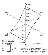
Test Conditions: Shock is applied in  $\pm X$ ,  $\pm Y$ , and  $\pm Z$  directions three times each with and without energizing the Relays to check the number of contact malfunctions.
