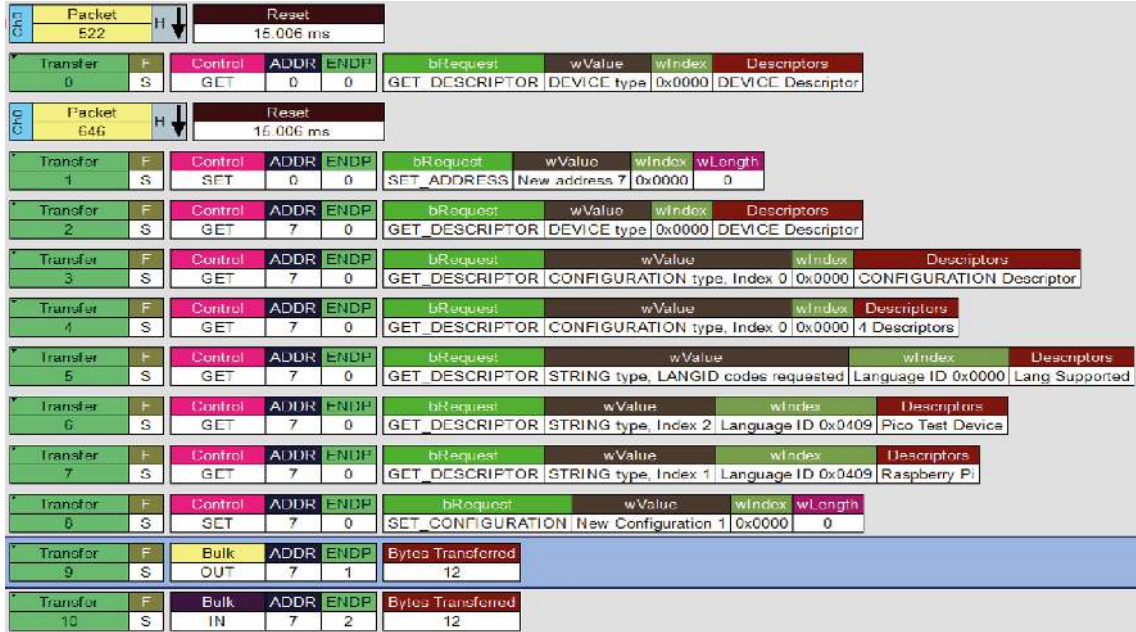
Figure 58. USB analyser trace of the dev_lowlevel USB device example. The control transfers are the device enumeration. The first bulk OUT (out from the host) transfer, highlighted in blue, is the host sending "Hello World" to the device. The second bulk transfer IN (in to the host), is the device returning "Hello World" to the host.
