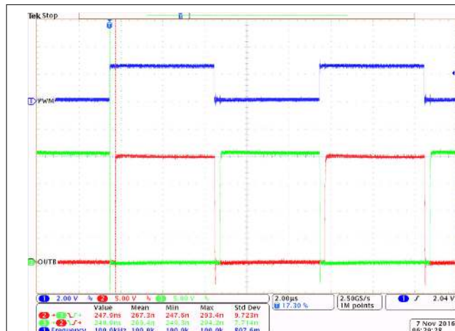
Figure 9-5. Bench Test Waveform for PWM and OUTA/B
