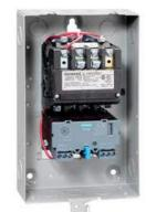
Non-reversing motor starter Size 1 Three phase full voltage Solid-state overload relay OLRelay amp range 0.75-3.4A 208VAC 60HZ coil Combination type Indoor general purpose use
