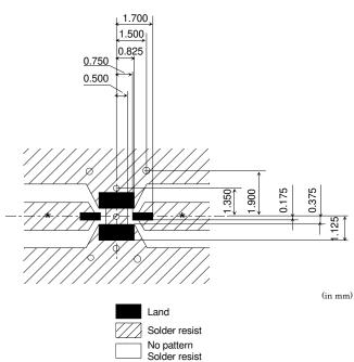
\* Line width to be designed to match 50 ohm characteristic impedance, Depending on PCB material and thickness.
