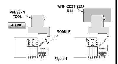
Reference: The 62203-0113 Press-In Tool is 16mm (0.63 in.) long.
