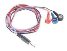
**Description:** This is your simple three conductor sensor cable with electrode pad leads. These cables are 24" long and feature a 3.5mm audio jack connector on one end with snap style receptacles for biomedical sensor pads. Each cable comes in a red/blue/black set.
