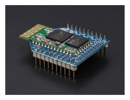
Bluetooth Bee is an easy to use Bluetooth SPP module compatible with existing Xbee sockets, designed for transparent wireless serial connection setup.
