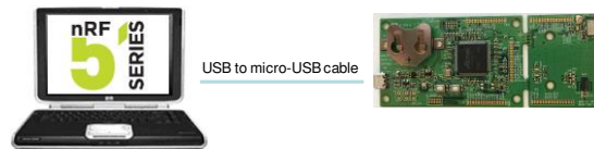
Figure 12 Configuration for application development with nRF52 SDK
