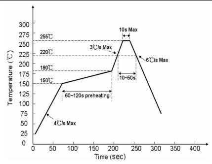
Note: Excessive soldering temperature and / or time might result in deformation of the LED lens or catastrophic failure of the LED.
