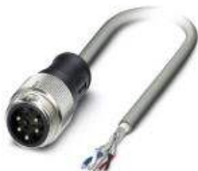
Bus system cable, DeviceNet, 5-position, PUR halogen-free, Gray RAL 7001, Plug straight 7/8"-16UNF, on Free cable end, Cable length: 5 m
