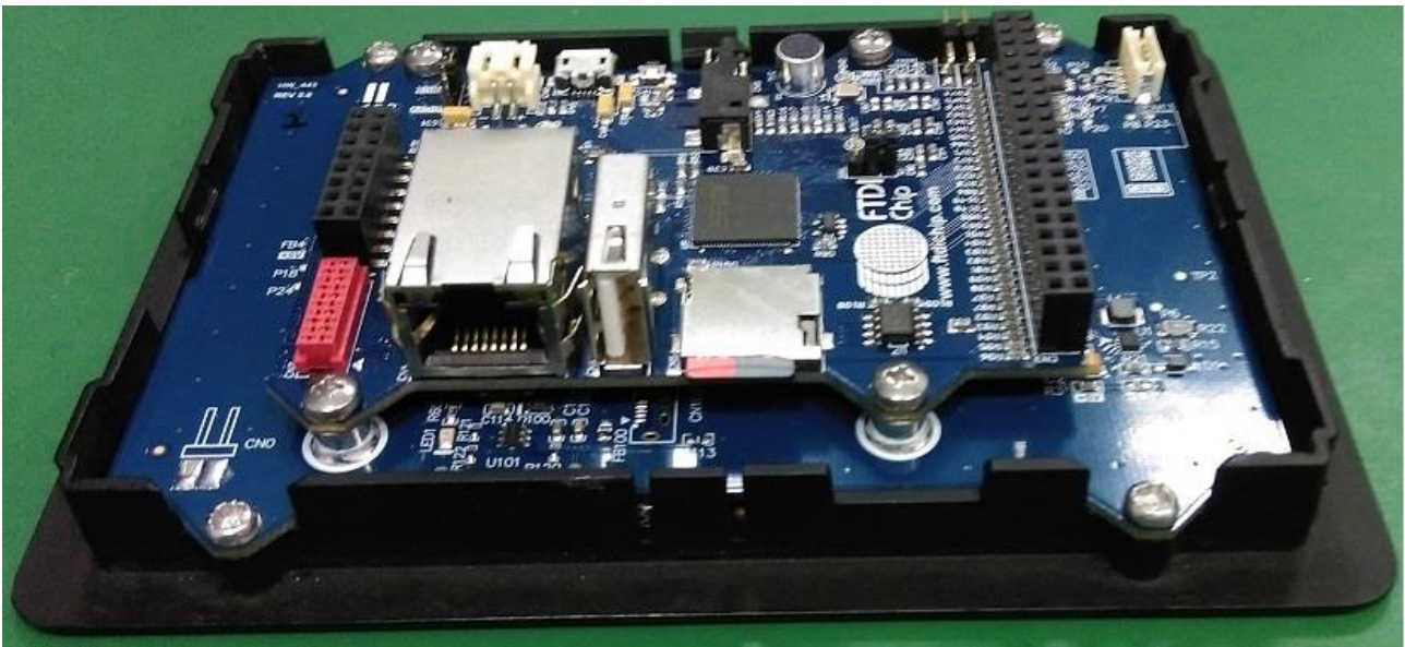
Figure 7-1 – ME812A-WH50R connects to MM900EV1A Module
