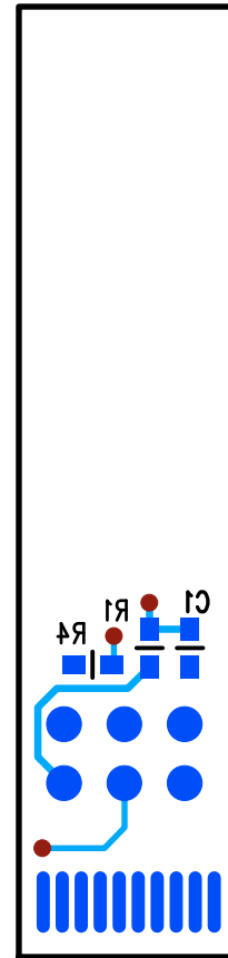
Figure 4-2. Bottom Layer + Silkscreen
