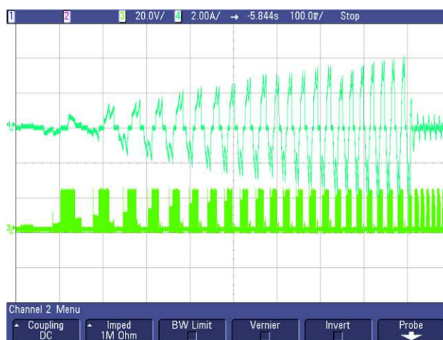
Figure 6. Open-Loop to Closed-Loop Threshold
