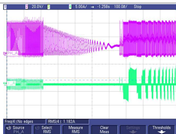
Figure 2. ISC Braking and Restarting Motor when Spinning in Reverse Direction
