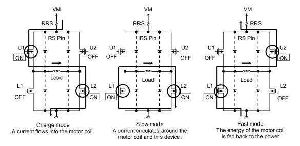
**Output transistor operational function**
