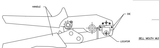
KEEP THE WIRE TO APPEAR KEEP THE INSULATION TO APPEAR BE SURE NOT TO ENCROACH ON THE WIRE BARREL SEAM MUST BE CLOSED WIRE MUST NOT BE EXPOSED BELL MOUTH MUST EXIST ROLLING ± 3'
