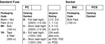
\*Note—Short lead length not available in tape-and-reel packaging. Note-Hi-Rel solderability applications should specify solder-dipped leads by adding -SD suffix to part number.
