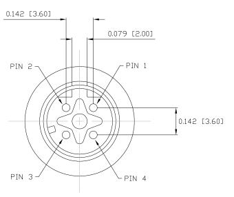
NOTE: MATERIAL HOUSING: PBT UL94V-0, BLACK CONTACT: BRASS NUT: BRASS □-RING: EPDM, BLACK SHELL: BRASS FINISH CONTACT: GOLD PLATED DVER 50u" NICKEL NUT: NICKEL PLATED SHELL: BRIGHT TIN PLATED ELECTRICAL RATED CURRENT: 4Α RATED VOLTAGE: 250V INSULATION RESISTANCE: 100 MOhms MIN. 10 m□hms MAX. CONTACT RESISTANCE: WATER PROOF: IP67 ENVIRONMENT OPERATION TEMPERATURE: -40°C T□ +85°C MAX WIRE AWG: 22
