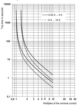
The time/current characteristic curve depends on the ambient temperatures. To avoid a premature or late switch-off, the nominal current of the circuit breaker must be multiplied with a temperature factor.
