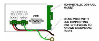
Both V- legs of the power input connector are connected to chassis internally on the PCB. Connecting a drain wire to earth ground from one of the V- terminal plugs as shown here will ground the switch and the chassis. The power leads from the power source should be limited to 3 meters or less in length.
