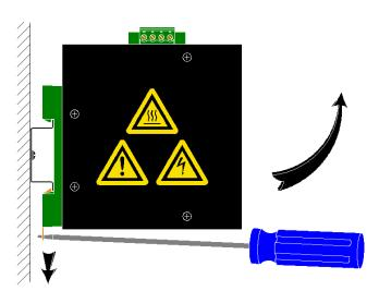
To remove the unit from the 35mm industrial DIN-Rail, place a flat head screwdriver into the orange release clip found at the bottom of the unit, and apply downward force on the clip until it disengages from the bottom of the unit from the DIN-Rail. Rotate the bottom of the unit towards you and up at an approximate 15° upward angle to completely remove the unit.
