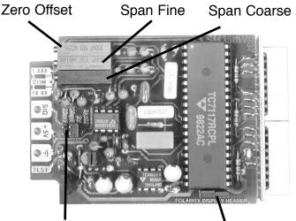
Range Select Header Polarity Display Header
