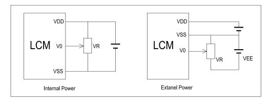
$V_{DD-}V_0$ : LCD Driving voltage VR: 10k~20k
