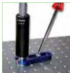
Mounting of Clamping fork (with Mounting column 14 on Holder A14) on Optical Table
