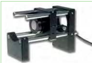
MT 25 as mirror positioner in microbench setup
