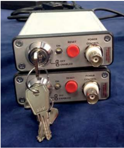
Photo shows 2 pcs. iFLEX-iRIS CDRH compliant interlocks and power supplies
