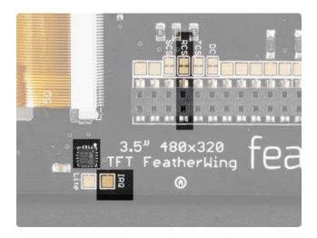
The touch screen also has a Chip Select line, labeled RT. This pin can theoretically be changed by cutting the jumper trance and soldering a small wire from the right-hand pad to the pin you'd like to use.
