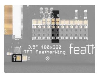
In addition, for the TFT display there is are D/C (Data/Command) and CS (Chip Select) pins. These are used to select the display and tell it what kind of data is being sent. These pins can theoretically be changed by cutting the jumper trace and soldering a small wire from the farther-from-the-socket-header pad to the pin you'd like to use.
