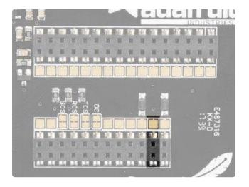
You can turn off the 3.3V power supply with the EN pin or the switch attached to that pin. The enable/disable switch on the bottom of the Wing will also deactivate the backlight
