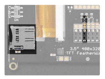
The SD Card also has a Chip Select line, labeled SD. This pin can theoretically be changed by cutting the jumper trance and soldering a small wire from the right-hand pad to the pin you'd like to use.
