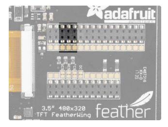
The TFT display, SD card and touch screen use the SPI interface to communicate. That means MISO, MOSI and SCK are used whenever either are accessed.
