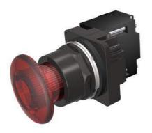
30mm BlackMax, Epoxy Coated Corrosion Resistant Complete Metal Unit Illuminated Push-Pull Operator Full Voltage, 120V AC/DC LED Lamp Mushroom Head Cap Small 1 3/4" (44.5 mm) Plastic, Red 3 Position Momentary UL Listed, CSA Certified NEMA 1,3,3R,4,4X,12,13 & Automotive Standards
