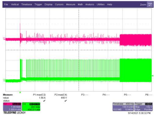
Figure 25 – Primary Clamp Drain Voltage and Current. 265 VAC, 5.0 V, 3 A Load (440 V MAX ). C4: V DRAIN , 200 V / div. C2: I DRAIN , 1 A / div. Time: 100 ms / div.
