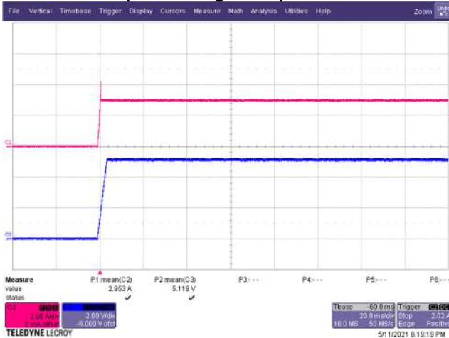
Figure 20 – Output Voltage and Current. 90 VAC, 5.0 V, 3 A Load . C2: I LOAD , 2 A / div. C3: V OUT , 2 V / div. Time: 20 ms / div.
