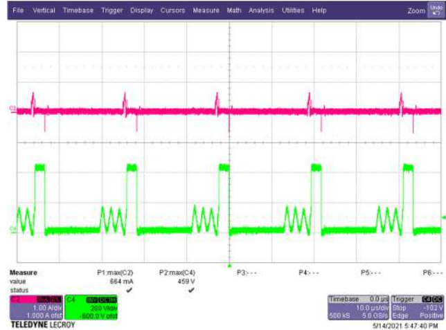
Figure 47 – Primary Clamp Drain Voltage and Current. 265 VAC, 9.0 V, 3 A Load (459 V MAX ). C4: V DRAIN , 200 V / div. C2: I DRAIN , 1 A / div. Time: 10 µs / div.
