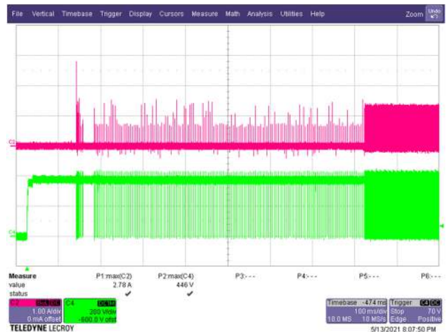
Figure 23 – Primary Drain Voltage and Current. 265 VAC, 5.0 V, 3 A Load (446 V MAX ). C4: V DRAIN , 200 V / div. C2: I DRAIN , 1 A / div. Time: 100 ms / div.
