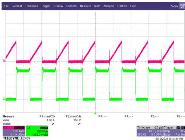
Figure 40 – Primary Drain Voltage and Current. 90 VAC, 15.0 V, 3 A Load (258 V MAX ). C4: V DRAIN , 100 V / div. C2: I DRAIN , 1 A / div. Time: 10 μs / div.
