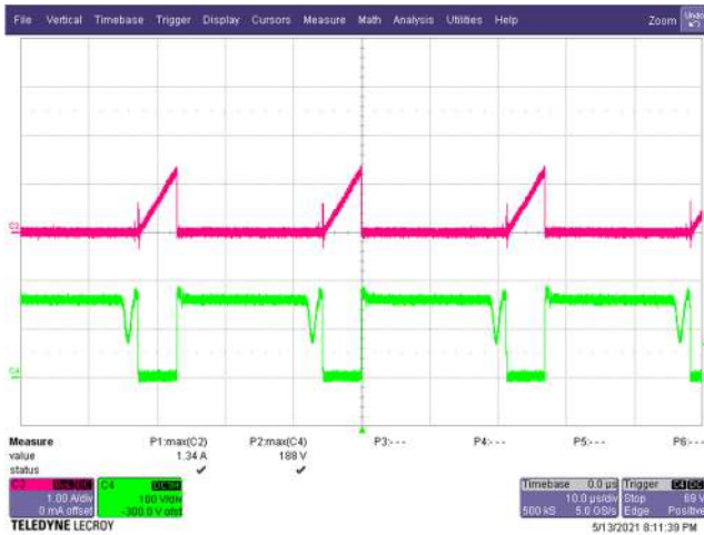
Figure 36 – Primary Drain Voltage and Current. 90 VAC, 5.0 V, 3 A Load (188 V MAX ). C4: V DRAIN , 100 V / div. C2: I DRAIN , 1 A / div. Time: 10 µs / div.
