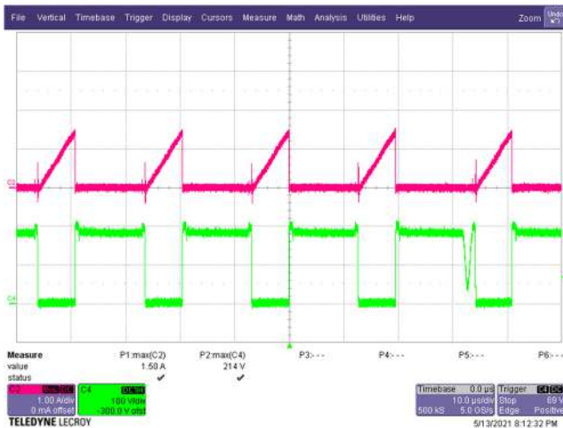
Figure 38 – Primary Drain Voltage and Current. 90 VAC, 9.0 V, 3 A Load (214 V MAX ). C4: V DRAIN , 100 V / div. C2: I DRAIN , 1 A / div. Time: 10 µs / div.
