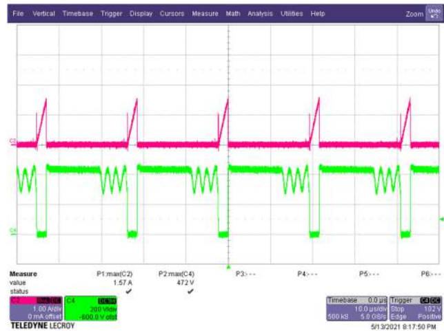
Figure 39 – Primary Drain Voltage and Current. 265 VAC, 9.0 V, 3 A Load (472 V MAX ). C4: V DRAIN , 200 V / div. C2: I DRAIN , 1 A / div. Time: 10 µs / div.
