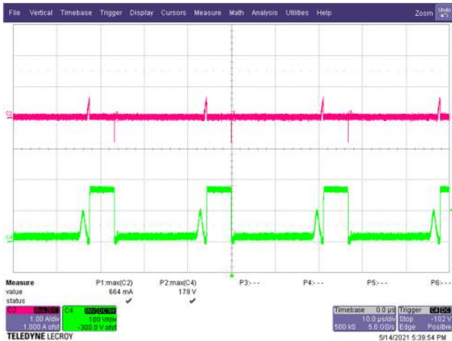
Figure 44 – Primary Clamp Drain Voltage and Current. 90 VAC, 5.0 V, 3 A Load (178 V MAX ). C4: V DRAIN , 100 V / div. C2: I DRAIN , 1 A / div. Time: 10 µs / div.
