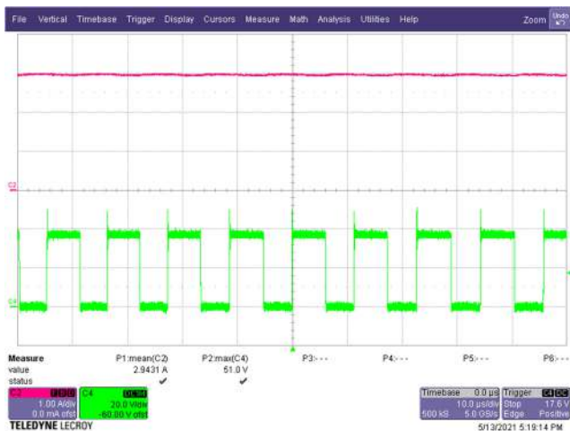
Figure 58 – SR FET Drain Voltage and Current. 90 VAC, 20.0 V, 3 A Load (51 V MAX ). C4: V DRAIN(SR) , 20 V / div. C2: I LOAD , 1 A / div. Time: 10 μs / div.
