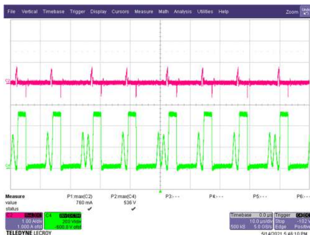
Figure 51 – Primary Clamp Drain Voltage and Current. 265 VAC, 20.0 V, 3 A Load (536 V MAX ). C4: V DRAIN , 200 V / div. C2: I DRAIN , 1 A / div. Time: 10 μs / div.
