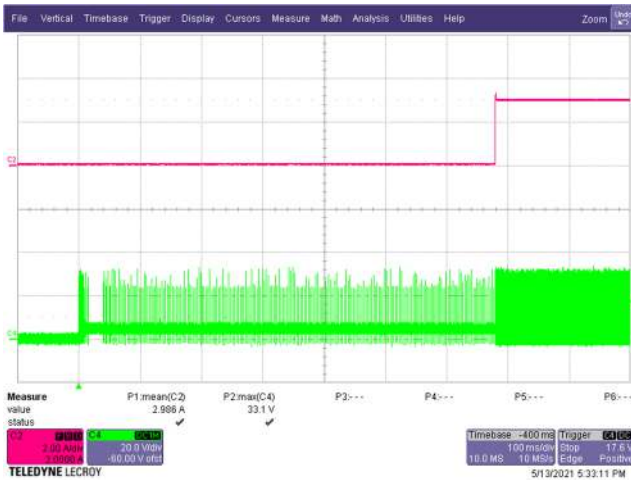
Figure 26 – SR FET Drain Voltage and Load Current. 90 VAC, 5.0 V, 3 A Load (33.1 V MAX ). C4: V DRAIN(SR) , 20 V / div. C2: I Load , 2 A / div. Time: 100 ms / div.
