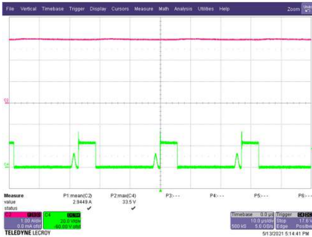
Figure 52 – SR FET Drain Voltage and Current. 90 VAC, 5.0 V, 3 A Load (33.5 V MAX ). C4: V DRAIN(SR) , 20 V / div. C2: I LOAD , 1 A / div. Time: 10 μs / div.
