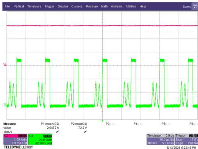
Figure 57 – SR FET Drain Voltage and Current. 265 VAC, 15.0 V, 3 A Load (72.2 V MAX ). C4: V DRAIN(SR) , 20 V / div. C2: I LOAD , 1 A / div. Time: 10 μs / div.
