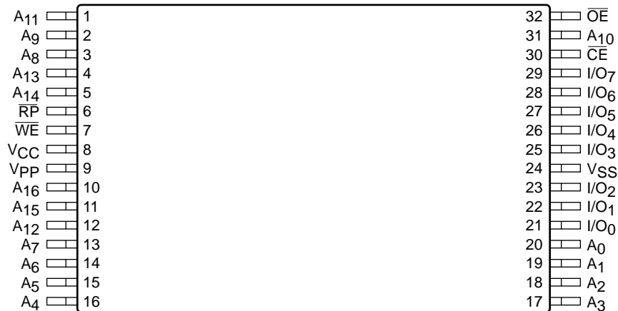
TSOP Package (Standard Pinout) (T, H)
