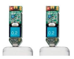
for connected devices, amounting to +/- 0.5 meters in typical situations. The result is a solution with 10x the accuracy of competing RSSI-based localization options.
