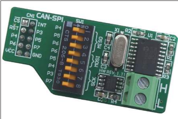
Figure 1: CAN-SPI additional board
