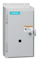
Non-reversing contactor, Size 2 1/2, Three phase full voltage, Contactor amp rating 60A, 3 wire (NO aux included), 190-220/220-240V 50/60Hz coil, Non-combination type, Enclosure NEMA type 12, Dust/drip proof for indoors, Standard width enclosure
