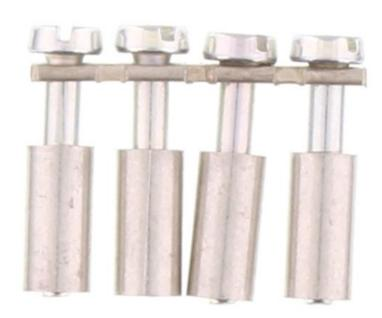
Cross-connector, No. of poles: 4, Mounting type: Can be screwed on, Width: 19.3 mm, Rated cross-section: 2.5 mm², Colour: natural
