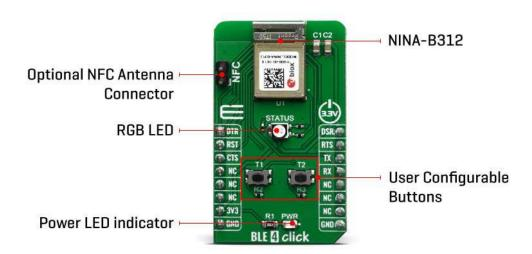
By integrating most of the critical components on the chip, the NINA-B312 allows the module to overcome any imperfections of external discrete components, allowing signal transmission power of up to 10dBm, and -94 dBm sensitivity for the receiver, using the on-chip antenna.
