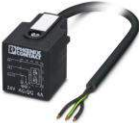
Sensor/Actuator cable, 3-position, PVC, Black RAL 9005, Free cable end, on A valve plug, with 1 LED, connected with Z diode, Cable length: 10 m
