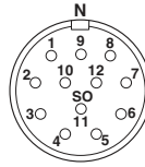
Pin assignment M23 socket, 12-pos., female side view
