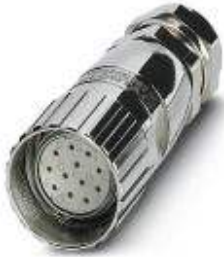
M23 socket, 12-pos., straight, freely configurable, with solder connection, for external cable diameter of 8 mm ... 12 mm
