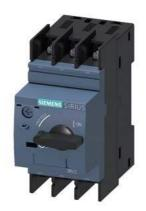
Circuit breaker size S00 for motor protection, CLASS 10 A-release 2.8...4 A N release 52 A ring cable lug connection Standard switching capacity
