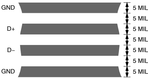
Figure 21. Typical Arrangement of Signal Tracks
