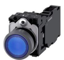
Illuminated pushbutton, 22 mm, round, plastic with metal front ring, blue, pushbutton, flat, momentary contact type, with holder, 1 NO+1 NC, LED module with integrated LED 110 V AC, screw terminal
