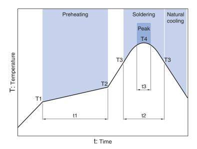
Preheating Soldering Peak Temp. Time Temp. Time Temp. Time T1 T2 Т3 **T4** t3 150°C 180°C 90 to 120s 230°C 255°C 40s 10s max.
