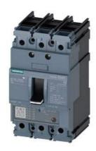
circuit breaker 3VA5 UL frame 125 3-pole, starter protection TM120M, AM, In=70A without overload protection short-circuit protection li=3...7 x In nut keeper kit on both sides
