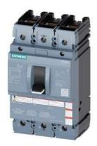
molded case switch 3VA5 UL frame 250 max. sh-circ breaking capacity 65kA @ 480 V 3-pole, line protection MCS110, ln=250A without overload protection self-protection li=10 x ln cable connection on both sides
