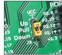
Figure 17-3: J9 in pull-down position
