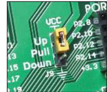
Figure 17-4: J9 in pull-up position
