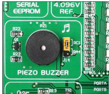
Figure 9-2: Signal generation via RC1
