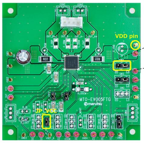
[Enlarged view of the jumper section]
