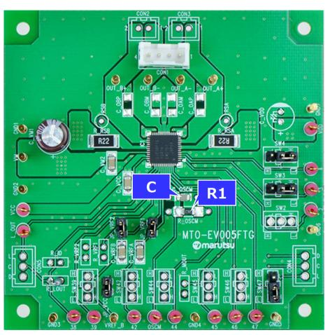
In PWM control of the TB67S103AFTG, the internal oscillation frequency (fOSCM) and the chopping frequency (fchop) can be adjusted according to the constant of the external components those are connected to the OSCM pin. In general,  $f_{chop}$  is recommended to set in the frequency range of 50kHz to 100kHz.
