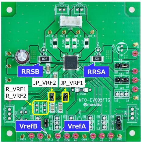
The TB67S103AFTG conducts motor operation by PWM constant current control which is based on the frequency of the OSCM oscillation circuit. The maximum current value (set Motor current value) can be determined by a sense resistor (RRS) and the reference voltage (Vref).
