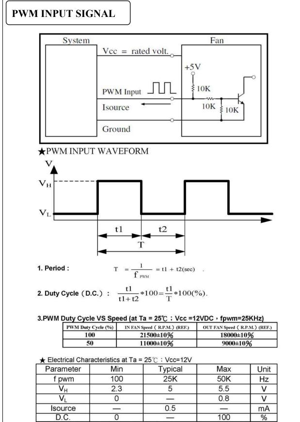
\* The speed is default to be maximum if PWM input pin is unconnected.
