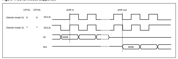
Figure 1. Serial Modes Supported
