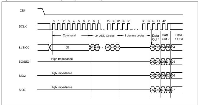
Figure 21. Quad Read Mode Sequence (Command 6B)
