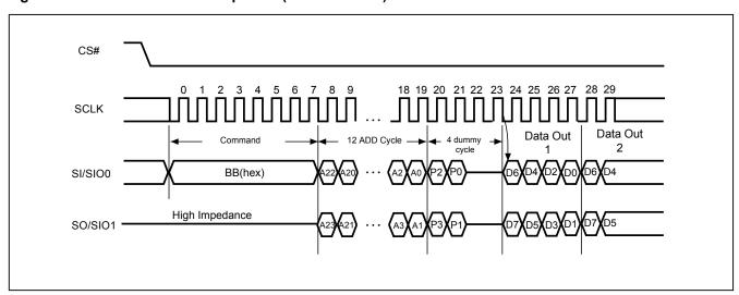
Figure 20. 2 x I/O Read Mode Sequence (Command BB)
