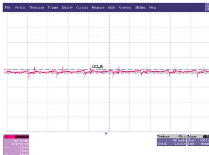
Figure 8. Buck Mode Output Ripple, VBUS = 5 V, VBAT = 3.7 V
