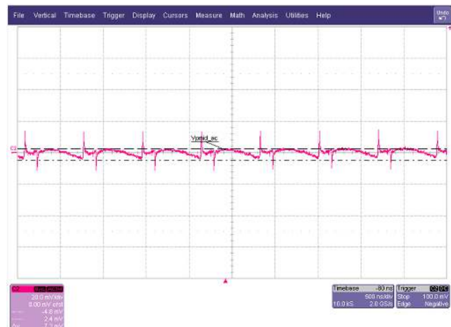
Figure 7. Buck Mode Input PMID Ripple, VBUS = 5 V, VBAT = 3.7 V
